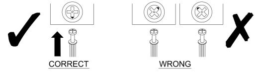
When fitting a cam lock, ensure the starting position is correct before inserting the connecting QUI CKFIT
