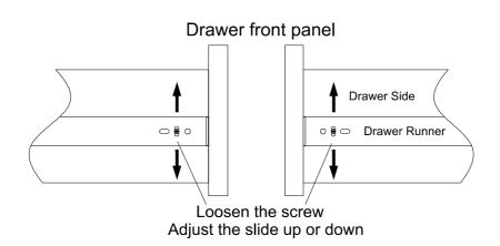
Loosen the screws on the left and right hand side, then adj ust the drawer slide up or down, untill the drawer fronts are even/level, then tighten the screws.
