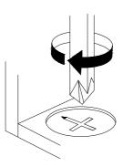
Turn cam lock clockwise to tighten.
