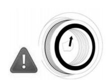
If you found the lamp won't illuminated after wire installed and inserted a E26/E27 light bulb, please try to raise up theintemal metal contactor in the socket.please make sure the power was disconnected before operated.
