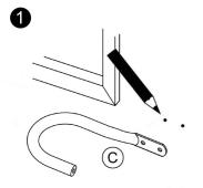
Use holdback (C) as a guide to mark location for mounting screws (A).
