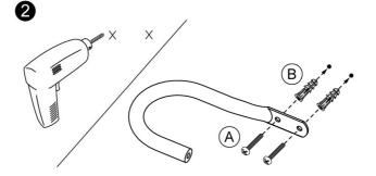
Drill pilot holes into wall with 1/4" drill bit (not included). Insert wall anchors (B) and attach holdback (C) using mounting screws (A). Wall anchors may not be necessary if drilling into studs.
