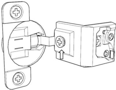
If the door is not level when it is installed, the customer will need to turn the screw clockwise to extend the hinge or counterclockwise to shorten the hinge.
