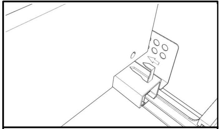
Ensure that the hook on each runner profile fits into the corresponding holes on the drawer back panel.
