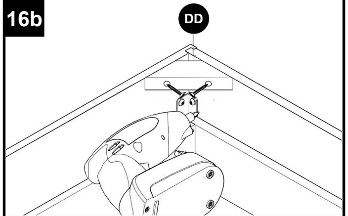
Use 1" flat head phillips screw x 8 (2 screws for 1 corner block)
