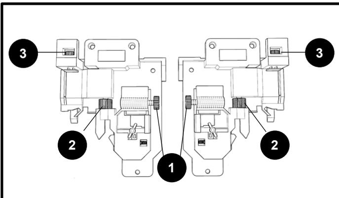
To level the drawer, use the green spur gears 1 to adjust drawer left and right, the green spur gears 2 to adjust drawer up and down, and the green spur gears 3 to adjust drawer inside and outside.
