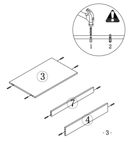
Strike the ¦Õ08\*40mm wood dowel pin into the ¦Õ8m hole of the above panels with an iron hammer. Please note that the hole of the three-in-one connecting rod should also be 8mm. The hole of the three-in-one connecting rod connects to the hole of ¦Õ15mm three-in-one eccentric wheel.
