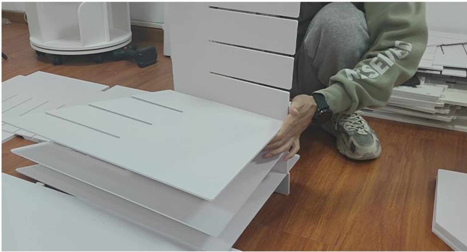
1. THE BOTTOM SLOT OF A-BOARD IS ASSEMBLED ON B BOARD IN TURN
