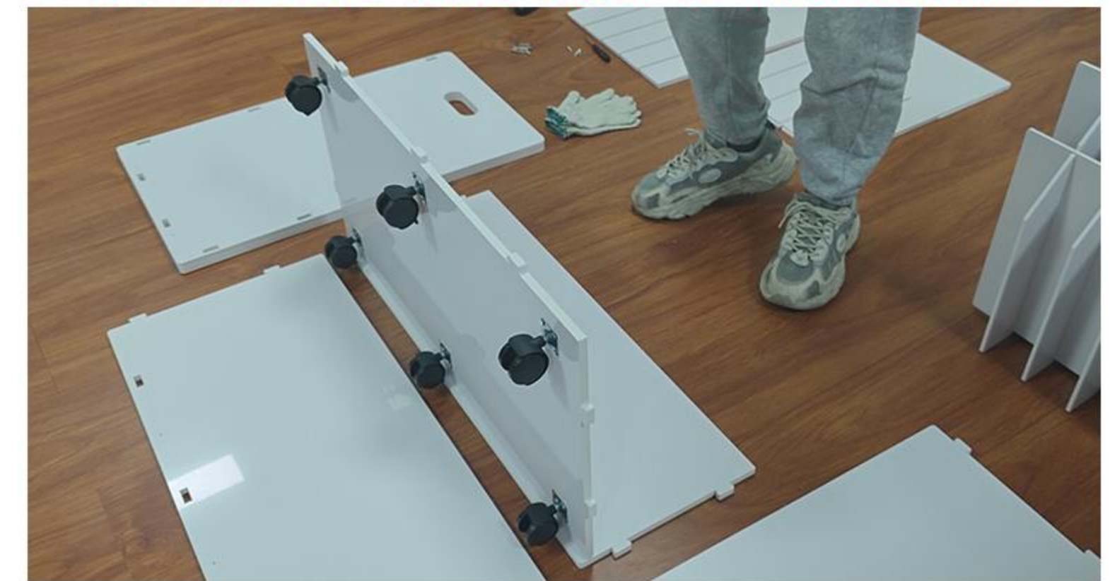
5. THE F PLATE IS ASSEMBLED ON THE G PLATE
