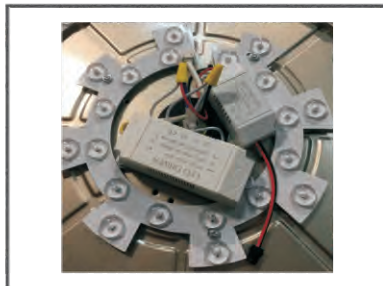
Step 3. Wiring diagram of LED light source and LED driver and Bluetooth driver.
