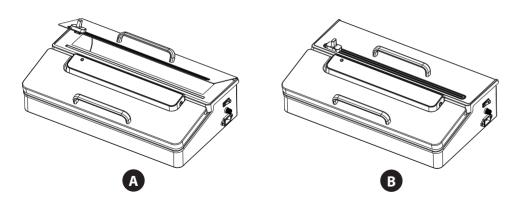
1. Open the roll lid, pull out the required length of Roll, then close the roll lid. Push the cutter button from left to right (as Picture B), then you can get any size bag you want. (**Note:** Do not need the cutter if it is vacuum bag instead of roll)
