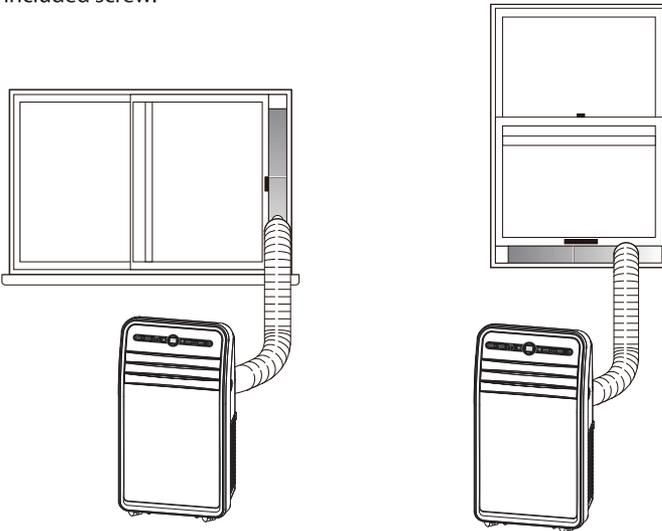
**Note:** For optimum performance, make sure the venting hose is not twisted and is free of kinks. For better efficiency, shorten the hose by squeezing its sections together.
