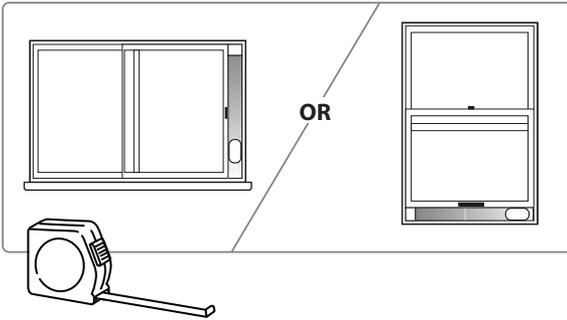
3. Install the window sealing plate in the window opening, adjusting the length to fit the window opening and securing it with "Clip" (provided).
