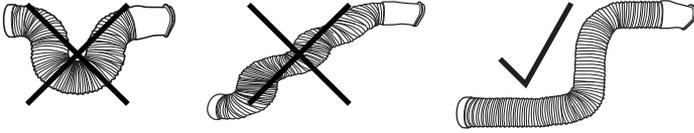
**Caution:** The exhaust duct is designed especially for this air conditioner. Replacing or lengthening the duct could result in damage to your unit.
