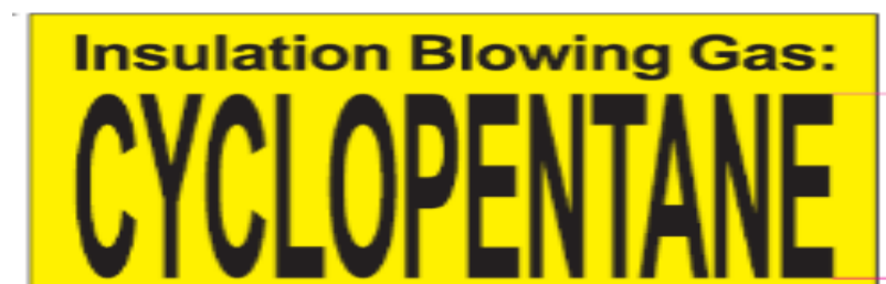
Illustration 1.2 - Marking for flammable insulation blowing gas type
