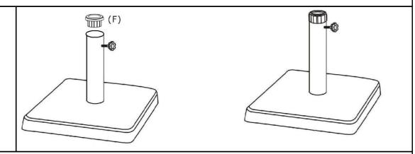
For the Umbrella pole with diameter as 48mm, use dia.48mm Adapter (F) only, insert the dia.48mm Adapter (F) into the Steel tube (B) to hold the Adapters in place.
