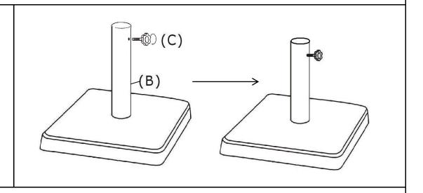
Screw Adjustable screw (C) into Support Pole (B).
