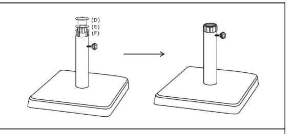
For the Umbrella pole with diameter as 35mm, use dia.35mm Adapter (D) & dia.38mm Adapter (E) & dia.48mm Adapter (F) added together, insert the dia.38mm Adapter (E) & dia.48mm Adapter (F) into the Support Pole (B) firstly, and then put the dia.35mm Adapter (D) onto the dia.38mm Adapter (E), to hold the Adapters in place. The Umbrella base is fully assembled and ready for use.
