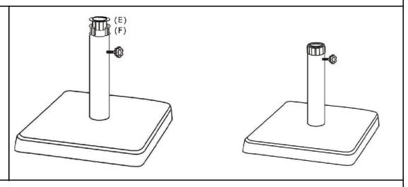
For the Umbrella pole with diameter as 38mm, use dia.38mm Adaper (E) & dia.48mm Adapter (F) added together, insert the dia.48mm Adapter (F) into the Steel tube (B) firstly, and then put the dia.38mm Adapter (E) onto the dia.48mm Adapter (F) to hold the Adapters in place.
