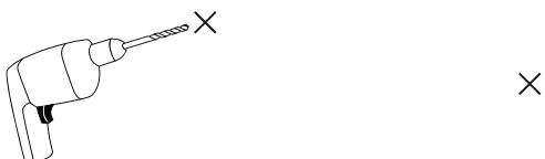
**3** Place shelf against wall, aligning the holes of the shelf & with the hole in the wall. Using a power drill or screwdriver (for Phillips head screw), drive provided screws through the shelf into studs or anchors.
