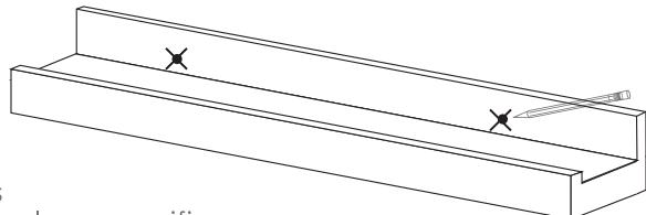
**2** Using a power drill and 9/32" drill bit, drill hole into wall marks. **Note:** If you are drilling into a wall where no studs are available, use the drywall anchors which have been provided.
