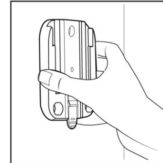
1. Determine mounting location for the light. Place the mounting plate on the surface so that the tab is pointing down, then mark the pilot holes. Be sure to leave at least 4 inches of clearance above the mounting plate so there is room to slide the light on.
