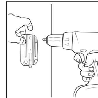
2. Use a 1/16" drill bit to create the pilot holes. If you are mounting to drywall, use the plastic anchors included with the screws. Use a hammer to tap the plastic anchors into the pilot holes before screwing in the mounting plate.
