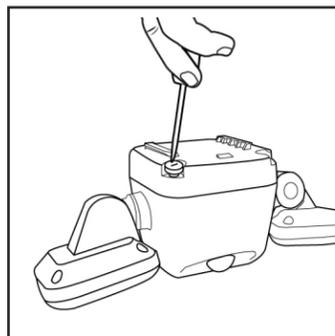
4. Replace the battery lid and twist the screws in tightly with a flat head screwdriver to activate the weatherproof seal.
