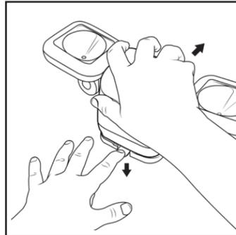
1. To remove the mounting plate from the light, press down on the mounting bracket tab. This will unlock the bracket. Slide the light off of the bracket while pressing down on the tab.
