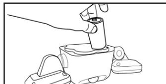
3. A) Insert 4 D-cell batteries. Ensure the batteries are inserted so that the flat ends are making contact with the springs. B) Choose a zone\* for your lights with the dipswitches next to the battery compartment. Ensure all units are on the same channel by matching the dipswitch positions on each light.
