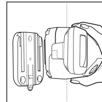
3. Line up the light with the mounting plate and slide the light into the grooves. Slide the light down until you hear it click into place.
