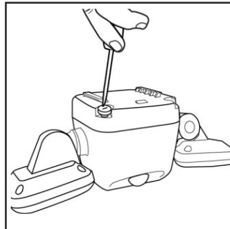
2. Use a flat head screwdriver or a quarter to loosen the four screws on the battery lid. **Note: The screws will stay attached.** Lift the battery lid off the back of the light.
