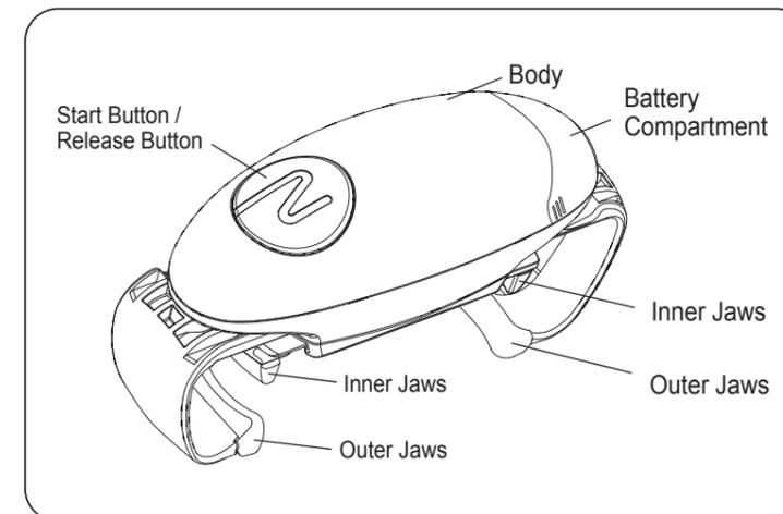
5. The Inner Jaws will grip the Jar Lid and then the Outer Jaws will resume their movement to hold the Jar securely. Then the Inner Jaw will rotate to open the jar lid.
