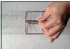
**STEP 8.2:** Insert the assembled glass tubes into the heater by holding the base in one hand, top in the other, and insert the tube underneath the flame screen (PART AA).
