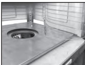
**STEP 8.3:** After inserting one side into the flame screen (PART AA), place the lower end on the rubber ring (PART DD) on top of the ceramic burner.
