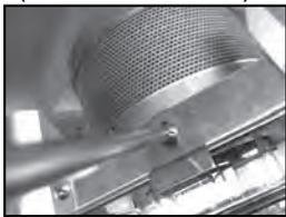
**STEP 11 :** Screw the knob with the chain (PART C) into the front panel and attach chain to the control box.
