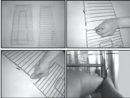
**STEP 10 :** Take guard fastening pieces from glass tube box. Screw the guard fastening pieces(PART D) on the top of the mounting plate to keep the screen firmly in place. (PARTB-4PCS )
