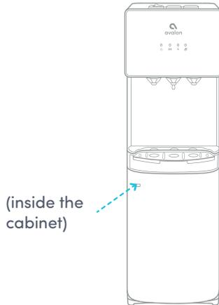
6. In order to flush the new filters, allow the water to flow from the cold water spout (#12) for approximately 2 minutes.
