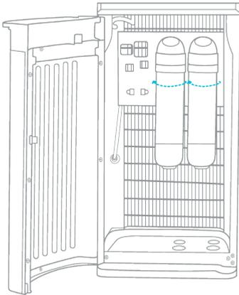
4. Turn on the Valve that was previously shut off. This Valve will be located at the connection to the water source or located to the left of the Sediment Filter.
