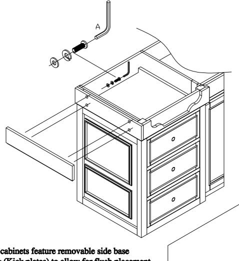
Note 1: cabinets feature removable side base moulding (Kick plates) to allow for flush placement against side walls and corners.
