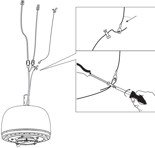
② Pass the cable through the down rod and lock the down rod.
