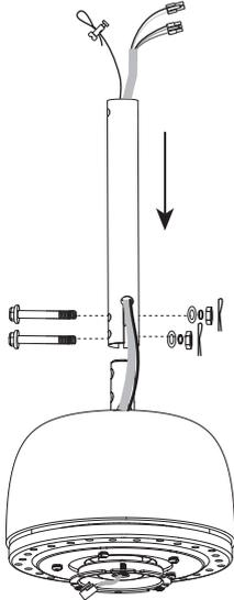
③ Install the Yoke cover and Canopy. Then insert the fixing pin, push the Hanging ball up, and fix it with screws.
