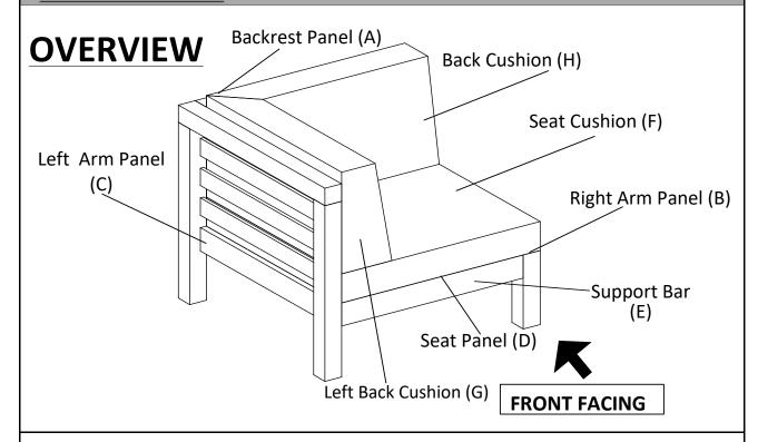
This Chair has multiple parts and may require up to 30 minutes to assemble. To give you an overview of the Chair parts, the above picture is to help you put the various parts into perspective. Please read through the instructions herebelow to familiarise the parts and steps before assembly.
