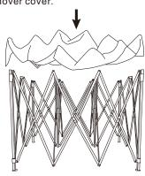
grasp the bottom of the diamond (shown), on opposite sides. Lift up and step backwards until shelter is fully opened, being careful not to pinch fingers.
