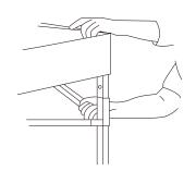
lift two adjacent outer legs up and pull out the inner legs until snap locks. Repeat on all legs. Raise or level the shelter using adjustment holes found near bottom of each outer legs.
