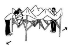
engage the auto slider at each corner by pushing up with one hand while holding down top of leg with the other hand. Snap botton will engage in groove. Repear on all other legs.
