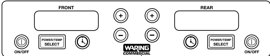
**NOTE:** This Induction Range requires induction-ready cookware. If the pan is not induction ready, it will not register on the induction range. The LCD display will show a flashing "STANDBY" when attempting to select a heat mode without an induction-ready pan on the glass cooking surface. The unit will automatically shut off after 60 seconds of not having an induction-ready pot/pan.
