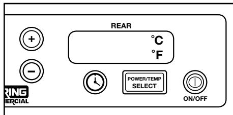
The screen will illuminate and display °C and °F, as seen above. The current setting will blink. Use the + and – buttons to switch to your desired setting. Once your desired setting is blinking, press the POWER/TEMP SELECT button to confirm, and then press the ON/OFF button.
