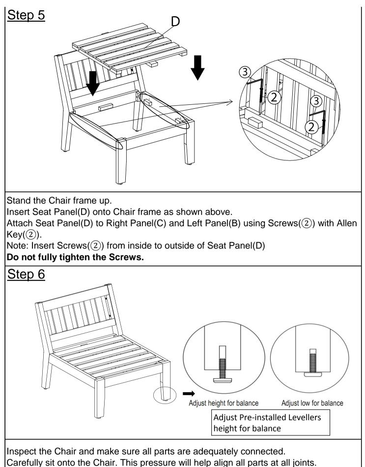
In a sequential manner, tighten all Bolts and Screws at all joints.
