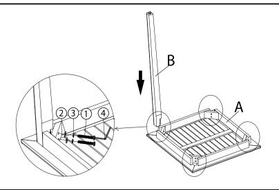
Place the Table Top(A) facedown onto a clean, non-marring surface. Attach Leg(B) into the mounting position at the corner of the Table Top(A) using Bolts(1), Washers(2), and Spring Washers(3) with Allen Key(4) as shown above. Repeat the same process with the remaining three Legs(B).
