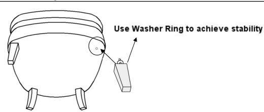
Install the Leg(B) into the Chair(A) by putting a Washer Ring(1) (improves tightness and security of leg)on the threaded stem.
