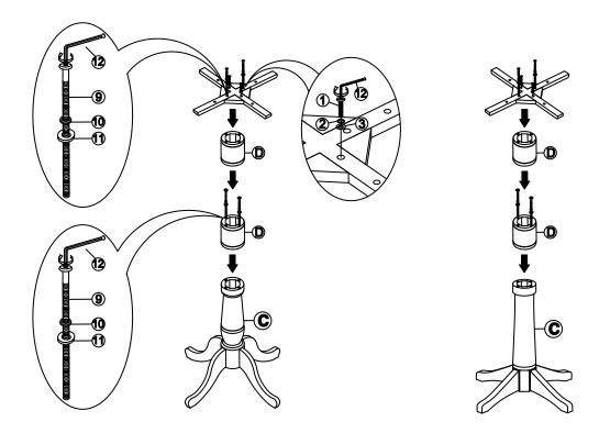
Attach the top (A) and pedestal extension (D) to the column (C) with long bolts (9), short bolts (1), washers (2), (3), (10) and (11) as shown below. Tighten with Allen key (12).
