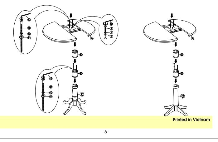
Attach mounting plate and pedestal extension (D) to the column (C) with long bolts (9), short bolts (1), washers (2), (4), (10) and (11) as shown below. Tighten with Allen key (12).
