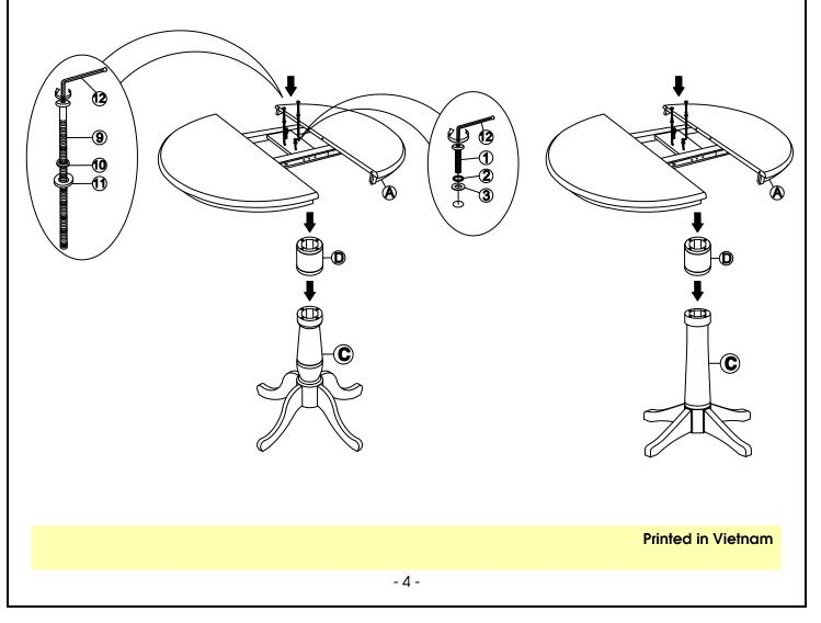
Attach mounting plate and pedestal extension (D) to the column (C) with long bolts (9), short bolts (1), washers (2), (4), (10) and (11) as shown below. Tighten with Allen key (12).
