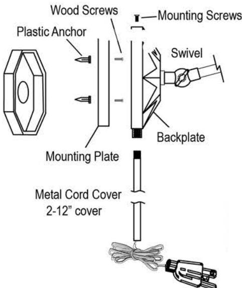
1. Use the plastic anchor and wood screws to mount the fixture onto the wall surface. The outlet box is not necessary for this application.
