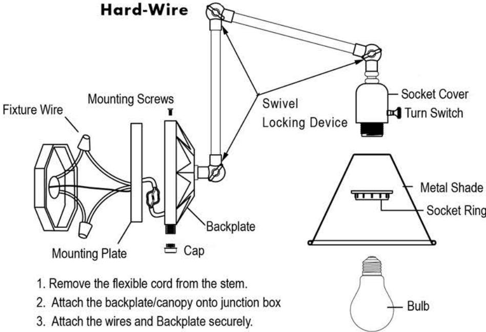
1. Remove the flexible cord from the stem.
