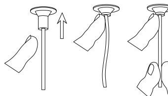
1.Using the tip of your finger or fingernail, depress the pin into the ceiling canopy, this will release the cable locking mechanism
