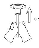
1.simply push up on the cable to raise the height of the fixture
