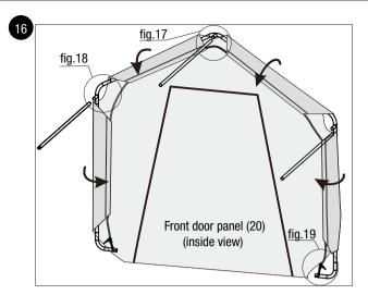
• Locate the top part of the front door panel (20) near the 3-way peak connector (11), disconnect the shoulder cross rail (4) from the 3-way peak connector (11), and pull the strap onto the connector (11). Then re-insert the cross rail (4) to its proper position (fig. 17).
