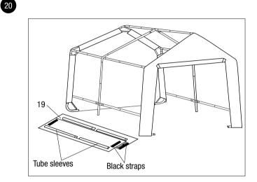
Stretch the roof tarp (19) over the shed frame and make sure it is center on the frame (fig. 21). Use a ladder if necessary.
