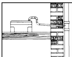
**CONNECTION TO DRAIN STACK PIPE**
