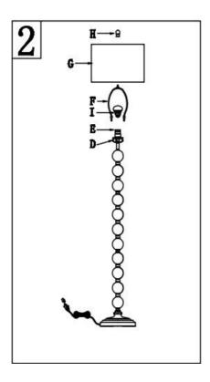
Insert the harp (F) into the saddle (D). Put the shade(G) on the harp(F),then tighten the finial (H)into the harp (F) Insert the bulb(I) into the socket(E).
