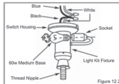
3. Carefully push all wires back into the switch housing. Then attach housing cover plate to switch housing with the 3 screws provided.
