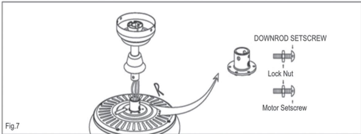
3. Tighten motor set screw. Check the strength of this connection (pre-tightened at factory) by holding the motor housing in position and turning the downrod counter-clockwise. If this connection slips, retighten motor setscrew and locknut. Follow the same procedures as mentioned above for downrod setscrew.
