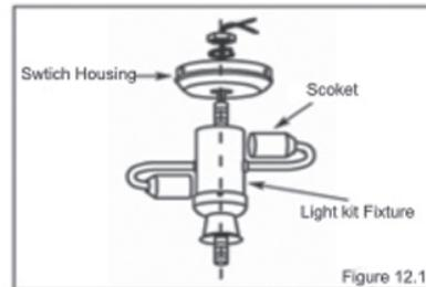
2. Locate two wires in the switch housing (white and blue labeled "for light").
