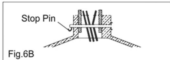
**WARNING:** Do not force connector pin through downrod. Use of force could cause damage to wires inside. Make sure the stop pin is properly engaged to prevent it from falling out.
