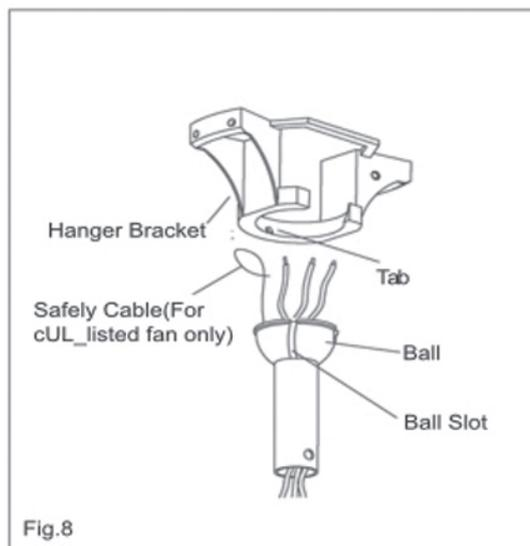
5. Make wire connections (refer to section titled “Electrical Connections”) **“For compliance with local codes and regulation. If installing the secondary support safety cable in the U.S., do not secure the safety cable within the outlet box!” You should mount the secondary support screw and cable outside the outlet box.**
