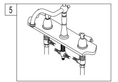
Connect the flexible tubes from the supply shank side port to the Spout Tee. Also reattach the supply lines, turn on the water supply, and check for leaks.
