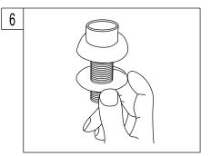
For model is with spray head and hose. Place the spray guide through the fourth hold in the sink, screw the locknut onto the shank and tighten firmly.
