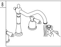
8. Remove the aerator before turning on your new faucet for the first time. Allow both hot and cold water to run for one minute. Replace aerator.
