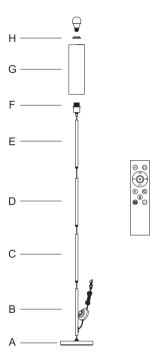
1.Screw the A-B-C-D-E-F parts together clockwise in turn as shown, and gently pull out the excess power cord from the bottom of the lamp base (B). 2.Place the shade (G) on the socket and screw the socket ring (H) to fix the shade.
