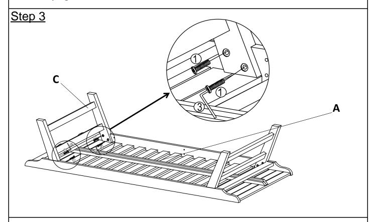
Attach the remanning Leg Frame(C) to Seat Panel(A) using Bolts(1) with Allen Key(3). **Do not fully tighten the Bolts.**
