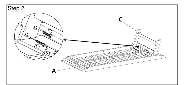
Place Seat Panel(A) facedown on a clean, non-marring surface. Attach Leg Frame(C) to Seat Panel(A) using Bolts(1) with Allen Key(3). **Do not fully tighten the Bolts.**
