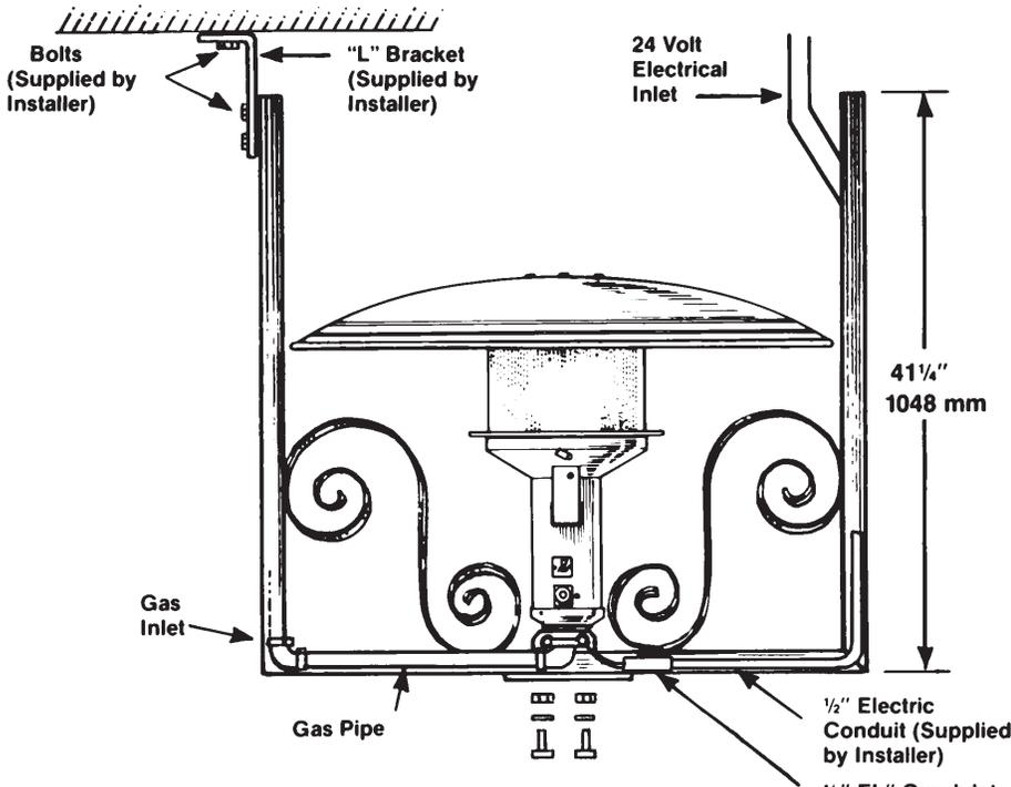
1. **Hanging Frame Mounting:** Before attaching the heater to the "U" shaped hanging frame, mount the frame in position to the overhead building structure. Use 3/8 inch diameter or larger bolts on each side leg. Position the frame to facilitate the connection of gas supply piping, and on models equipped with an electrical valve, the electrical supply wiring.
