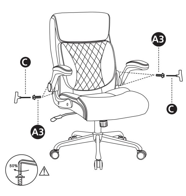
Step 7: Then Tighten All the Screw by 100%.
