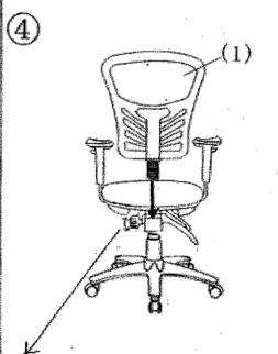
Insert the back into the mechanism and adjust to desired height, turn the button counter-clockwise until it is screwed in tightly.
