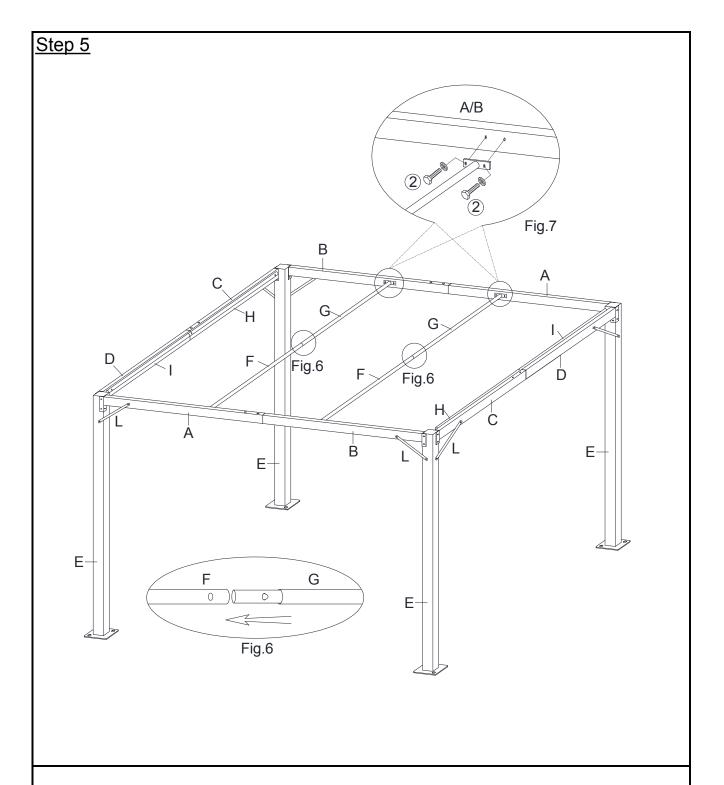
Attach Supporting Fabric Tubes(F) to Supporting Fabric Tubes(G) using the preattached snap buttons. (See Fig.6)
