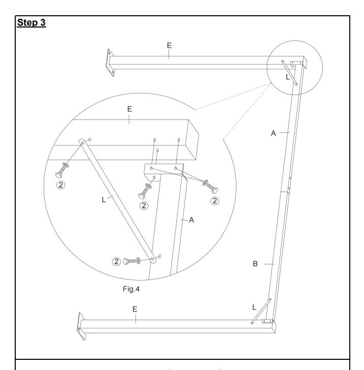
Attach Crossbars(A) to Main Pillars(E) using Bolts(2) with Wrench(3).
