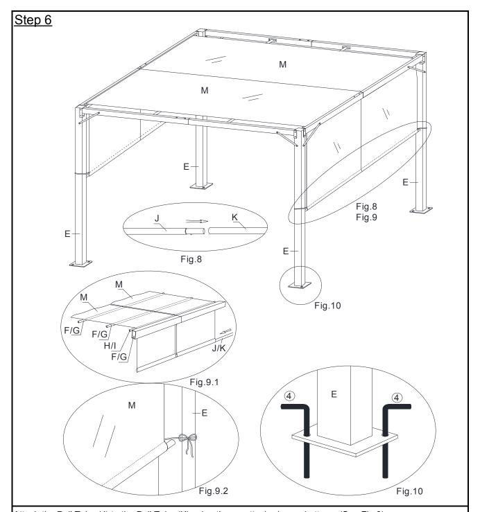
Attach the Pull Tube (J) to the Pull Tube (K) using the preattached snap buttons. (See Fig.8) Insert the Canopy(M) through Supporting Fabric Tubes(H/I), then onto Supporting Fabric Tubes(F/G). Insert the Pull Tubes(J/K) into the sleeves of the Canopy(M).
