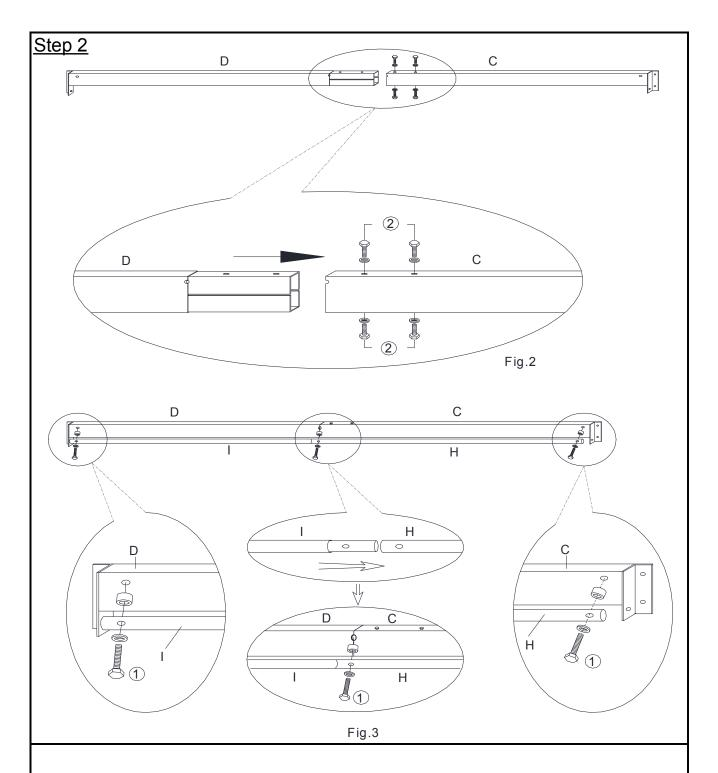
Attach Crossbars(C) to Crossbars(D) using Bolts(2) with Wrench(3). (See Fig. 2)
