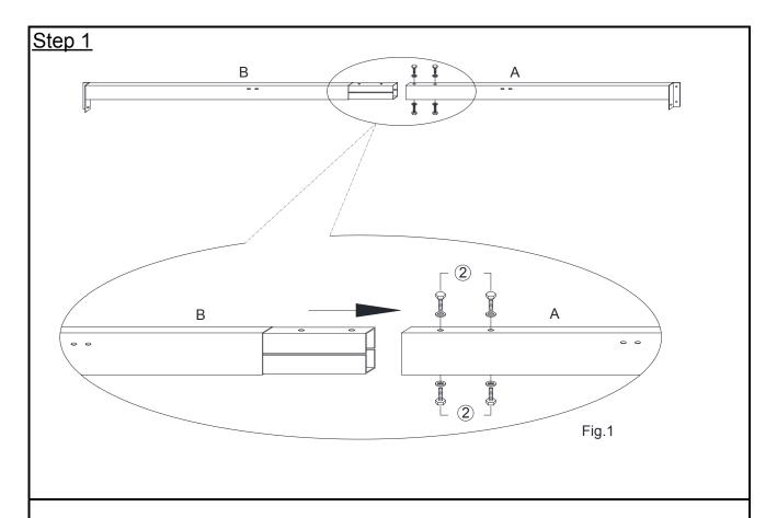
Attach Crossbars(A) to Crossbars(B) using Bolts(②) with Wrench(③). (See Fig. 1)
