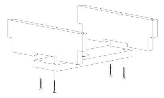
Note: The bottom support board should **\*NOT\*** sit flush with bottom of the side supports:
