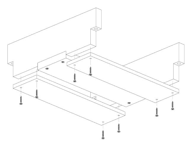
NOTE: There should be a small gap between the boards – this is normal and is designed to help with drainage
