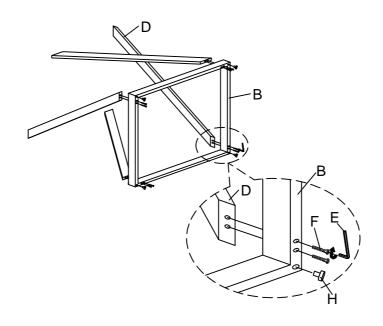
2 Attach the upper frame (A) to the cross bars (D), using the bolts (G) and L-allen key (E) to tighten.
