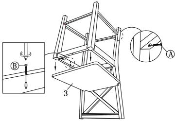
There are No Pre-Drilled holes to attach the seat
