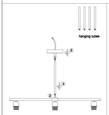
2.Let the wire go through the hanging tube4, rotae to fasten the tube on the fixture 2 (connect more tubes to get suitable heighten), let the wire go through canopy 5, turn to fasten the canopy 5 on the fixture.
