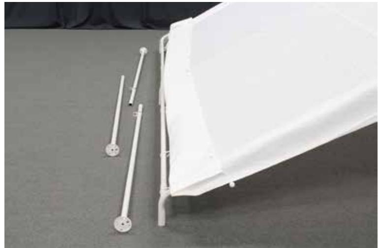
**7)** Next continue attaching the straps down each side and end. Make sure the cover stays centered on the frame.
