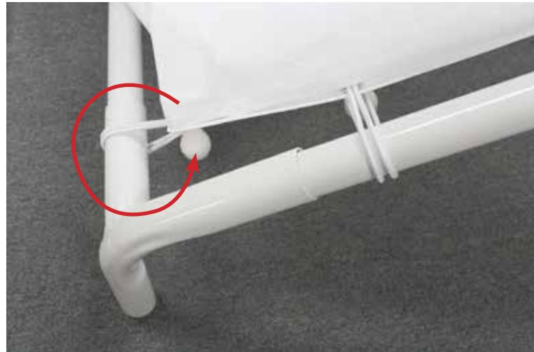
**4)** Wrap the cord around the pole and secure around the ball.
