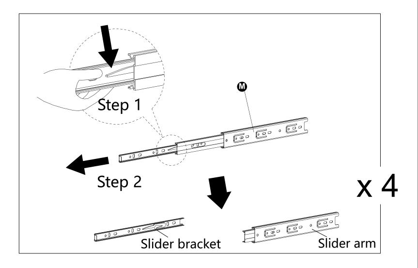
· Separate the slide bracket from the slide arm as per diagram.
