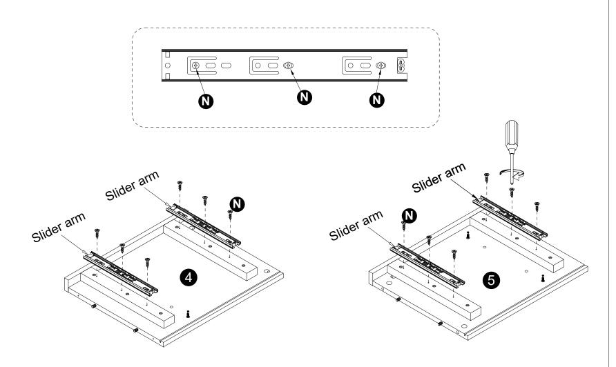
· Attach slider arms to panels (4,5) with screws (N) correctly.
