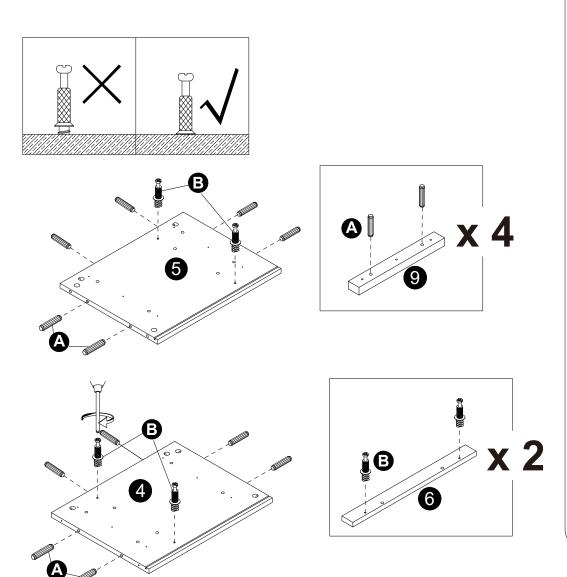
•The provided glue(H) is to secure When first inserting dowels, locate the wood dowels(A) in place. appropriate hole for the dowel, place a small amount of glue in the hole and insert the dowel.
