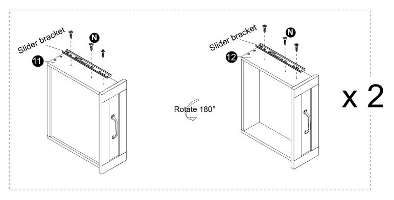
· Attach slider brackets to panels (11,12) with screws (N) correctly.
