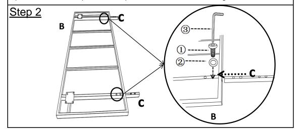
Turn the Table Top Right(B) face down on a clean, non-marring surface. Attach Support Bar(C) to Table Top Right(B) using Bolts(1) and Washers(2) with Allen Key(3).
