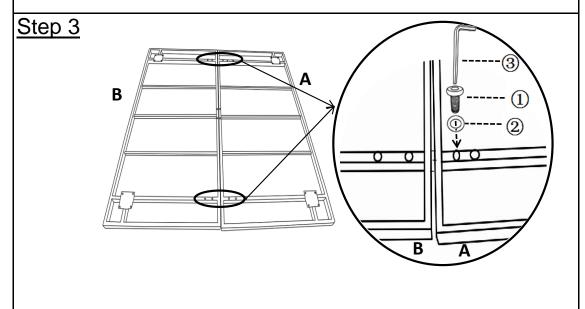
Repeat Step 2 ,Attach Support Bar(C) to Table Top(A) using Bolts(1) and Washers(2) with Allen Key(3).
