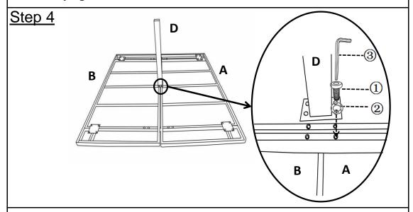
Attach Table Middle Leg (D) to Table Top(A)&Table Top (B) using Bolts(1) and Washers(2) with Allen Key(3).
