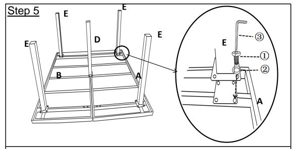
Attach Table leg (E) to Table Top(A)&Table Top (B) using Bolts(1) and Washers(2) with Allen Key(3).
