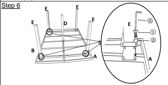
Repeat Step 5 to assemble balance Table Legs(E), using Bolts(1) and Washers(2) with Allen Key(3).
