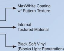
PVC/Woven Screen Material, Multi-Layer, Cross-Array Layout, Coated with Matte White Optical Material that is Mildew Resistant.
