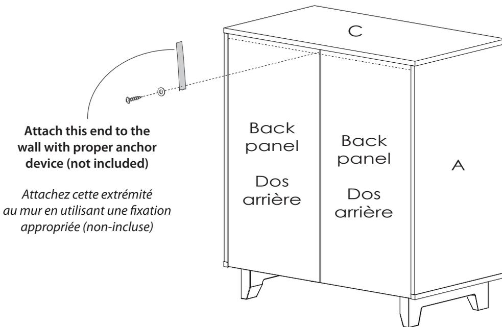
**Attach this end to the wall with proper anchor device (not included)**
