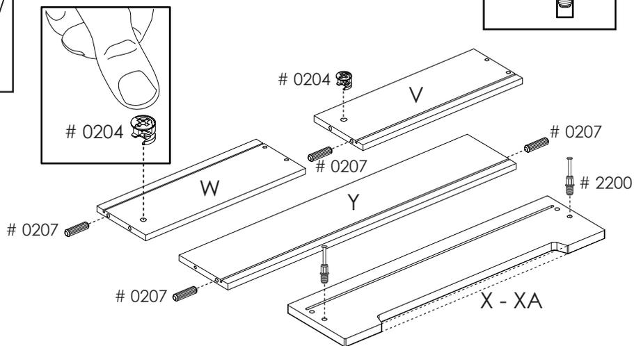
**11** Fasten the panels V and W to the drawer front X or XA and tighten the 2 cam locks # 0204
