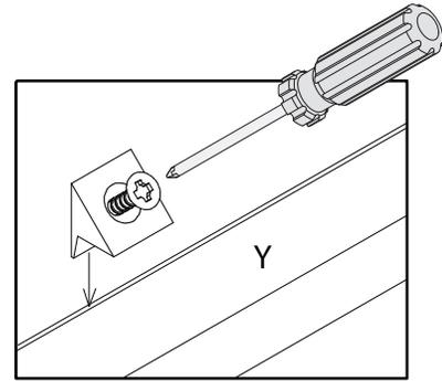
**Insert the small lip of the connector into the groove. Then, hold firmly the connector and screw in place**
