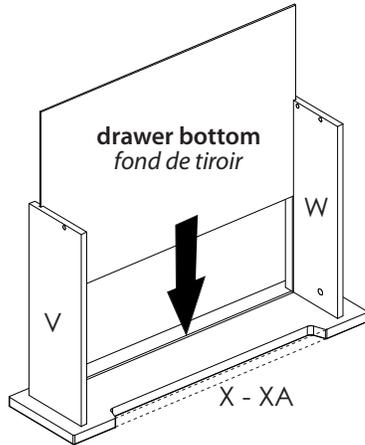
**Drawer bottom must enter into the groove located on panel X or XA**
