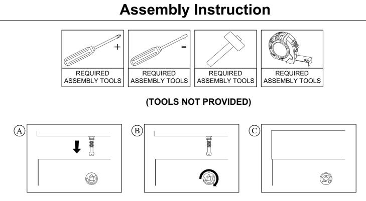
Use a screwdriver to tighten the cam nuts as the sequence above. A quarter turn clockwise is all that is needed.
