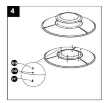
Attach reflector assembly to head assembly (C).
