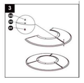
Attach reflector plate (B) to reflector panels (A) using M6 x 8mm screws (FF), Φ6 washers (DD) and cap nuts (GG).
