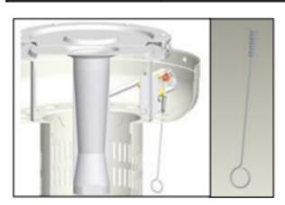
If for some reasons your ignition fails to deliver a spark, the heater can be started by inserting a lit match using supplied match holder through the burner hole (see left photo) while pushing the control knob in the "PILOT" position, which shall be performed by a qualified person
