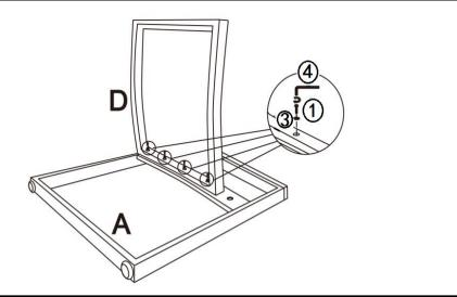
Open the carton and place all the parts onto a clean, non-marring surface. Attach Seat(D) to Left Armrest/Leg(A) using Bolts(1) and Washers(3) with Allen Key(4) as shown above.
